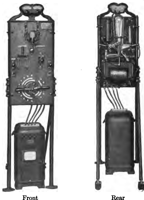
FIG. 349. Front and rear views of a General Electric mercury-arc rectifying outfit for charging storage batteries.
